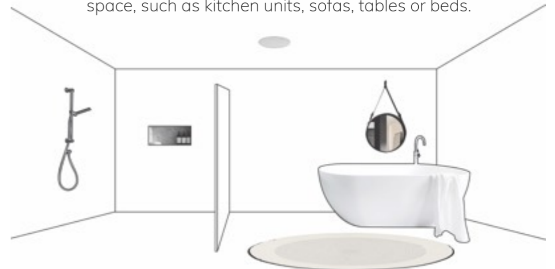
In small rooms such as bathrooms it may be necessary to use a single-stereo speaker rather than a stereo pair. Ensure speakers aren't positioned directly above a shower cubicle or bath unless they have IP66 certification.
